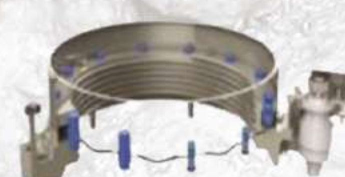
液压驱动锁紧 Hydraulically Driven Locking
